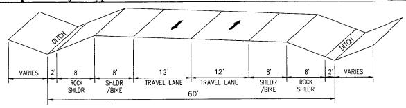
Typical section will vary, including a two-lane rural cross-section and two-lanes with a center turn lane at intersections.
