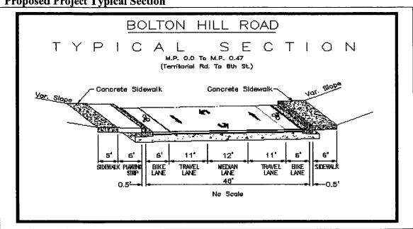
Note: Two basic types of typical sections proposed for 3-lane and 2-lane roadways. MP 0.47 to MP 0.65 is proposed for two lanes.
